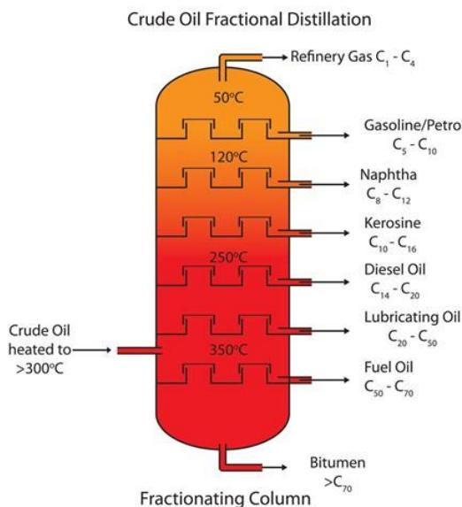
There are several ways of classifying the useful fractions that are distilled from crude oil. One general way is by dividing into three categories: light, middle, and heavy fractions. Heavier components condense at higher temperatures and are removed at the bottom of the column. The
